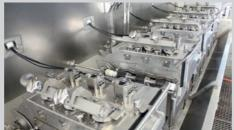
Thanks to its exclusive piezo-electric linear actuator, the MCD3 offers an unequalled range of space-dyeing effects:
