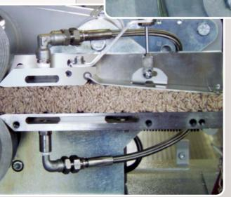
> Adjustment of the desired frieze effect is achieved through a pneumatic jack controlled by PLC
