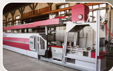
MAT3 can be installed on the floor or on top of the heat-setting line.
