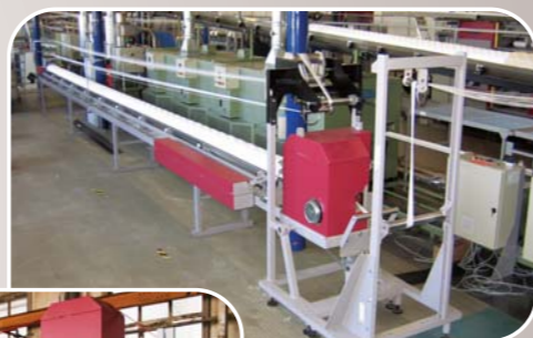
MAT3 can be installed on the floor or on top of the heat-setting line.
