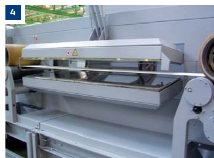
Heating plates with more power for higher shrinkage.
